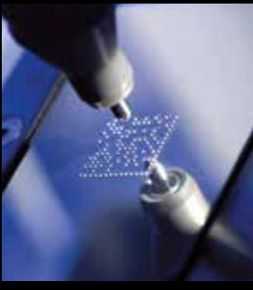
Dot peen marking
